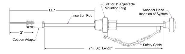
**Model SR3000** coupon insertion system is an adjustable unit commonly used in the water treating industry. The system is designed to mount onto a 1" piping system, but can easily be adapted to fit your specific requirements. The system consists of an insertion rod with a coupon adapter. The standard assembly is available with 3/4" or 1" NPT threads on the mounting plug. A safety cable and safety nut are also provided to prevent blowout. Several coupon holders and lengths are available.
